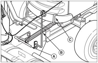
Figure 21. Lift Assist Spring
